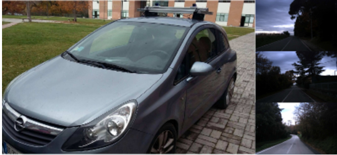
Fig. 7: Car setup used for collecting the Perugia Countryside Dataset. On the right, some sample images of the recorded sequences are shown.
